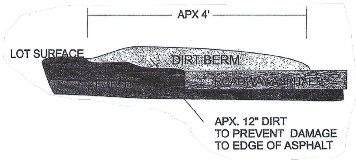
Dirt berm should be placed wherever vehicles will access the property and will remain in place until the driveway apron is complete or until such time as no construction vehicles will be assessing the property.
